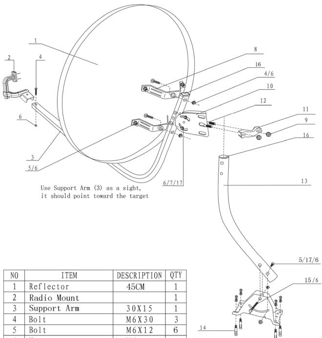
Nut M 6 6 12 M6X45 2 Bo1t Reflector Mount 2 2 Nut M8 Adjustable Mount 10 1 11 Pipe Clamp 1 U-Bolt 12 M 8 1 Stand Pipe Φ42 13 1 14 Anchor Bolt M6X504 15 Bo1t M6X60 1 16 Plastic Cover 2 4 17 Washer Ф6
