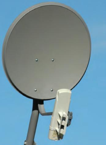
(Above) MoWiNet Reflector using Motorola Canopy
